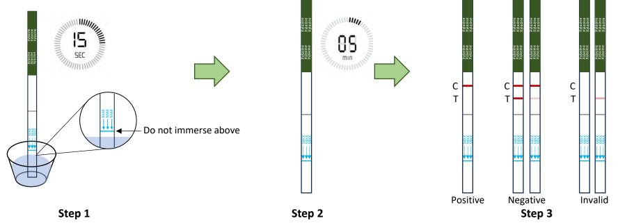
Dip the strip in the liquid and hold for 15-20 Take the strip out and place it on a non-seconds. You should see liquid migrating up.
